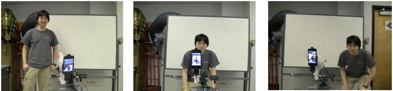
a) GunBot tracking target's left movement b) GunBot locked into the target c) GunBot tracking target's right movement
