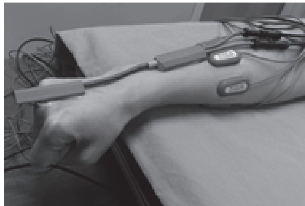
Figure 1. The experimental set-up. The one electro-goniometer was placed on dorsum of hand and forearm (long green rod). Six sEMG active electrodes were placed around middle forearm.
