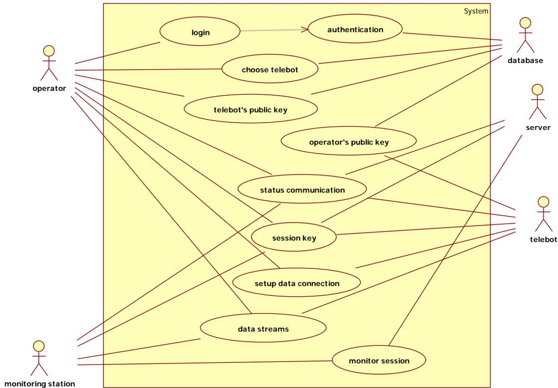
Fig.3 UML Use Case Diagram
