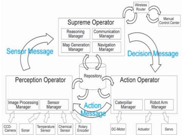
Fig. 2: Operational architecture of the robot
