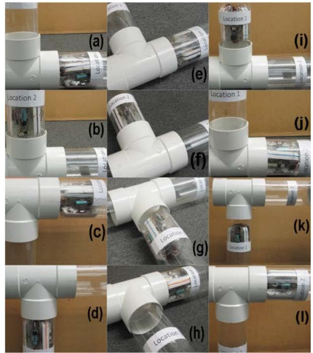
Fig. 14: Types of motion at T-branch, where (a)-(d) show H to V, (e)-(h) show H to H, and (i)-(l) show V to H motion
