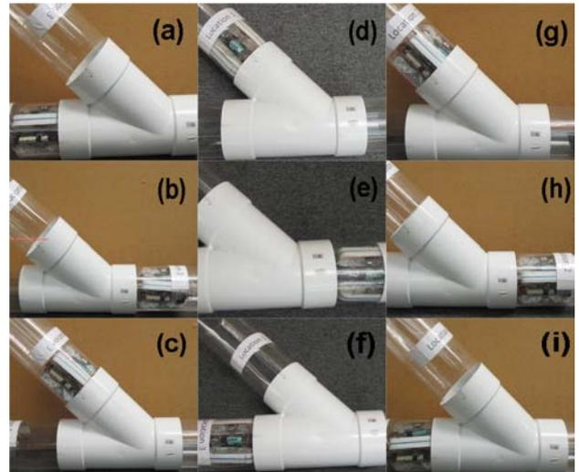
Fig. 15: Types of motion at Y-branch, where (a)-(c) show H to V, (d)-(f) show H to H, and (g)-(i) show V to H motion
