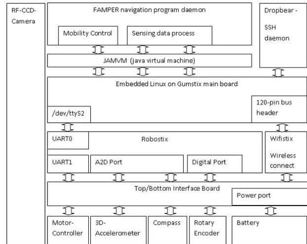
Fig. 11: Electrical architecture of the robot
