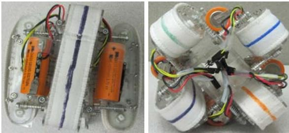
Fig. 17: The 5 degrees tilted caterpillar-based robot design
