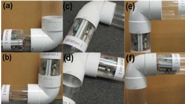
Fig. 13: Types of motion at 90 degrees elbow, where (a), (b) show H to V, (c), (d) show H to H, and (e), (f) show V to H motion
