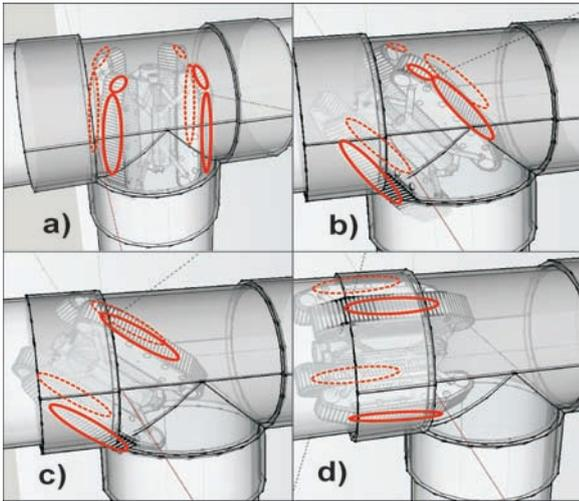
Fig. 8: Depiction of the pipeline surface contact by robot wheels at T-branch
