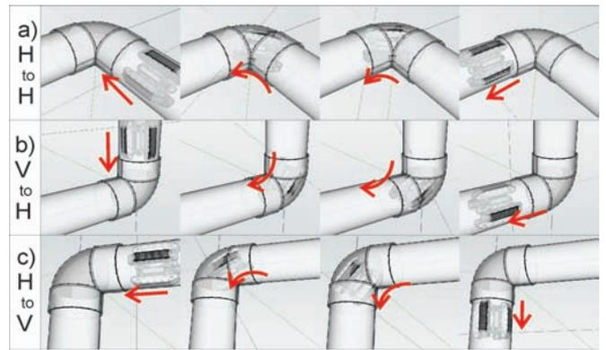
Fig. 6: Motion planning at 90 degrees elbow, where H to H indicates Horizontal to Horizontal, V to H indicates Vertical to Horizontal, and H to V indicates Horizontal to Vertical motion
