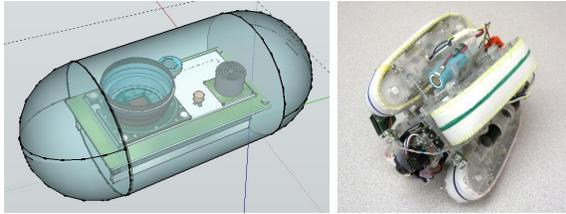
(a) Mobile sensor (HPMS) design (b) Robot agent FAMPER
