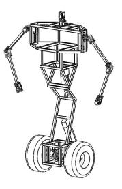
Fig. 1b TeleBot lightweight metal wire frame angled to maintain TeleBot shape
