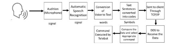
Fig. 9 Block diagram of TCP/IP and Free TTS based Greeting/Control system of TeleBot
