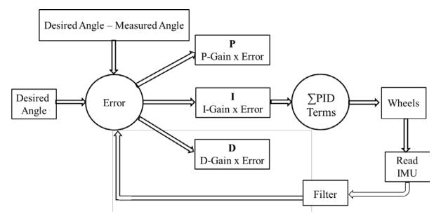
Fig. 7 Block diagram of the PID Controller
