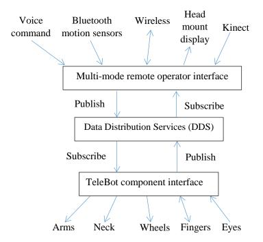
Fig. 6 TeleBot Communication Architecture/Control System
