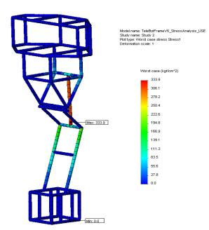
Fig. 2 Weight on upper TeleBot frame - stress analysis of worst case scenario
