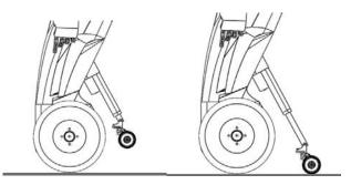
Fig. 4aRetracted linear actuator while TeleBot is in motion on flat ground
