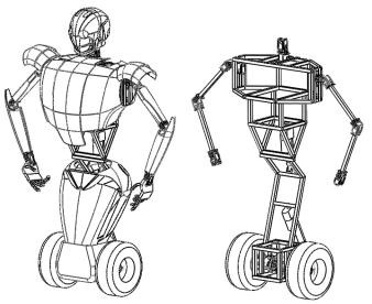
Fig. 3aModified physical TeleBot exterior with framefor the real world
