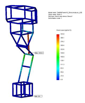
Fig. 6 Weight on upper TeleBot frame – stress analysis of worst case scenario
